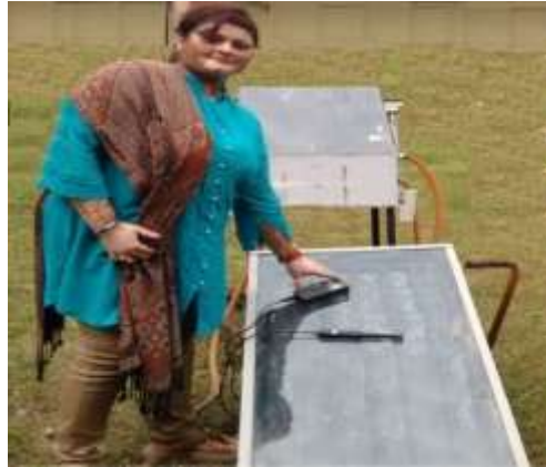
Fig 1: Experimental setup of solar still (23°) with collector
